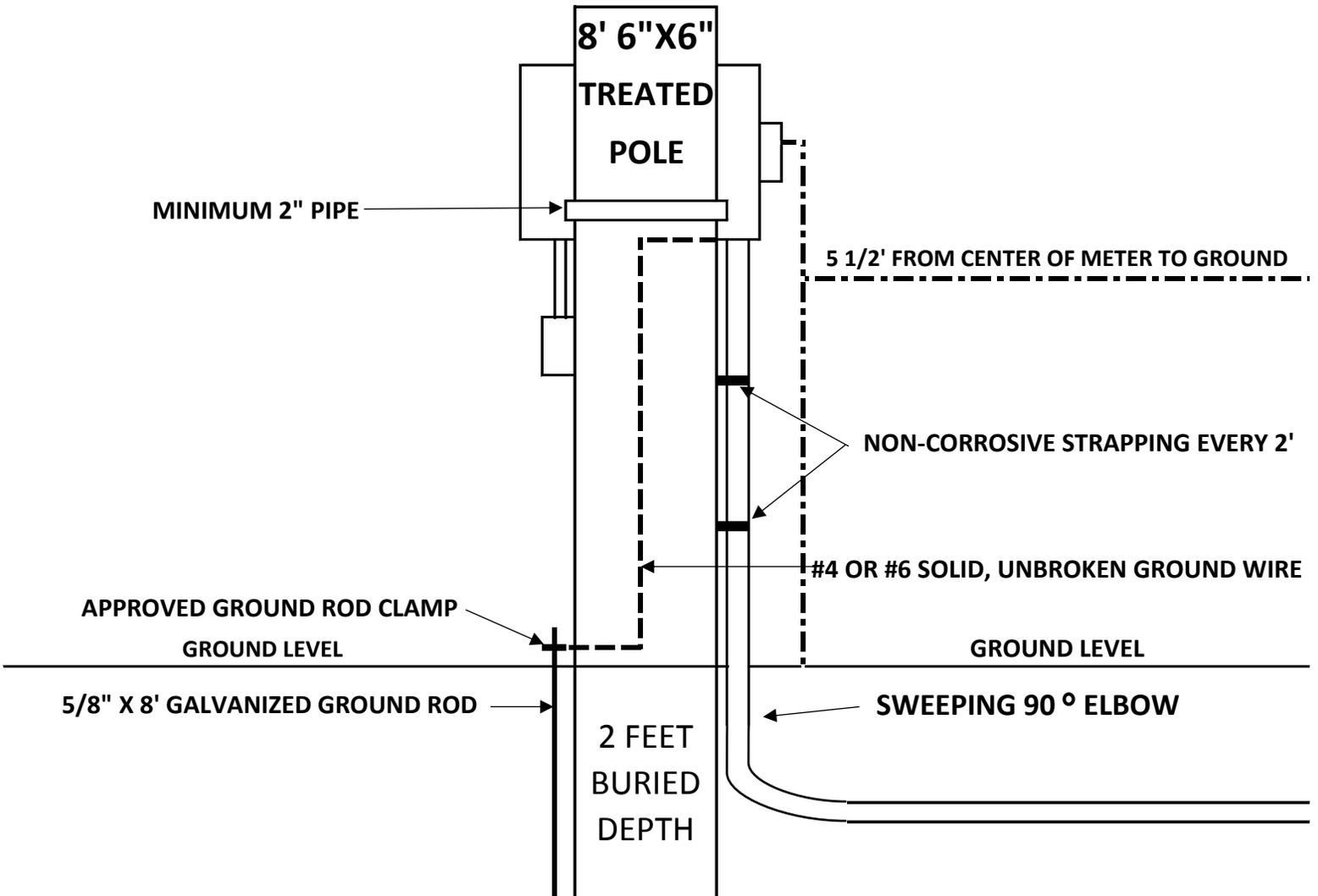
All wiring must meet State of Tennessee wiring code and the National Electric Code (NEC). T.V.E.C. will not connect to a meter pole until approved by Tennessee deputy state inspector
